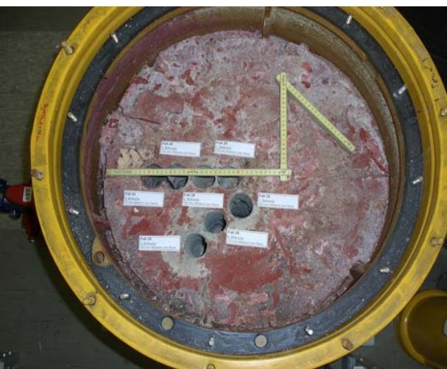
after approaching steady state (with respect to solution composition) termination & core drilling
